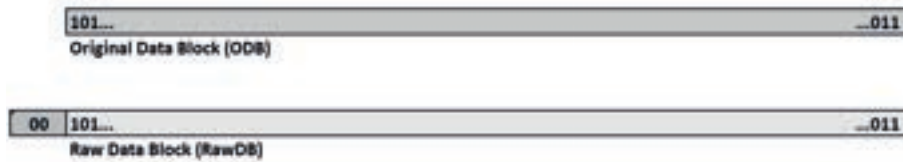
Figure 2. Original Data Block (ODB) with n bit length is transformed into Raw Data Block (RawDB) by creating a RawDBH header consisting of '00' and attaching original data of n bit ODB in unchanged form.
